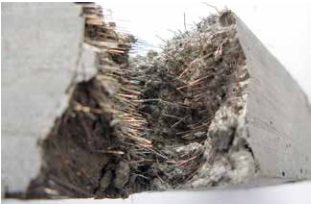
High strength and above all ultra high strength concrete are practically always also fiber-reinforced. Depending on the requirements, synthetic and/or steel fibers are thereby employed in large quantity. The high flexural strength of UHPC can be achieved in this way.
