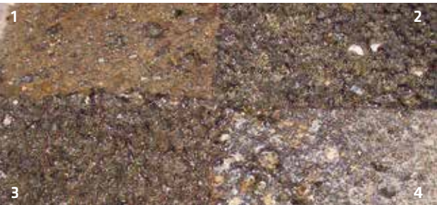
Fire exposure trials for concrete containing various aggregates. Surface spalling and sintering, and a range of temperature developments at differing depths can thereby be compared.
