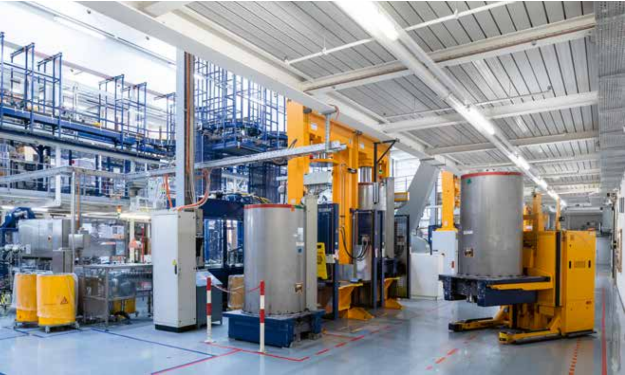
Sika's adhesives production in Dürdingen, Switzerland, is fully automated – from the preparation of starting materials, through the production and filling of cartridges to the packaging and palletizing of the end products.
